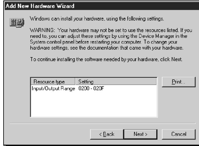
Figure 2-10 I/O Range Assigned to the NIC Screen
